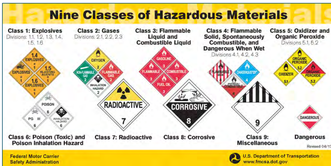
Figure 5: US DOT Placards for Hazardous Materials Classifications
