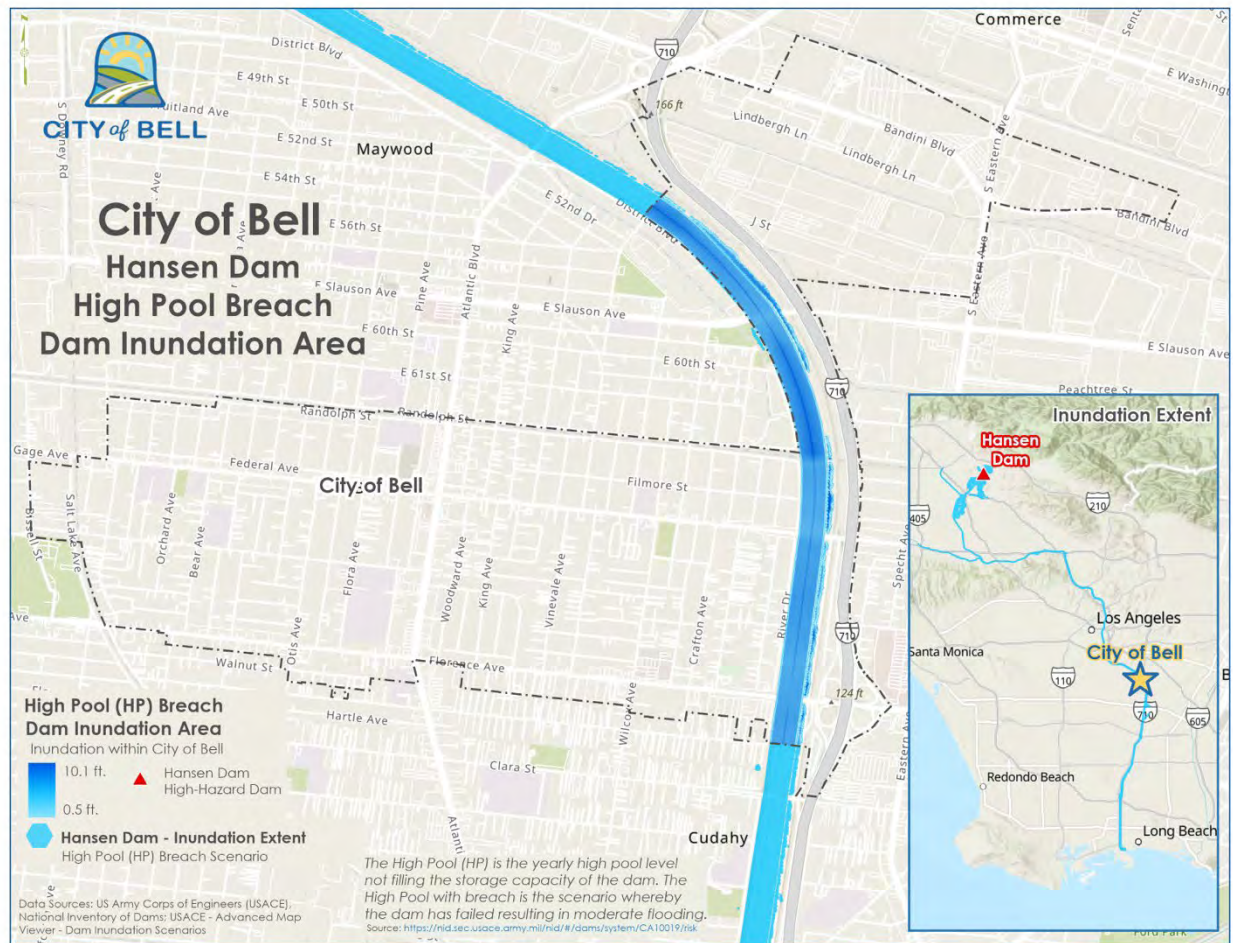
Figure 11. Hansen Dam Inundation Area – High Pool Breach
